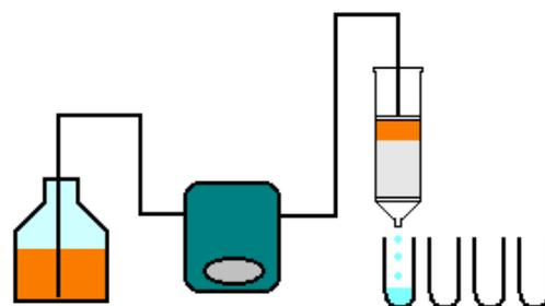
Up to the fraction No.8, the Pd was removed completely. After then, the column reached a breakthrough point and the drain showed a same concentration with the former solution.
