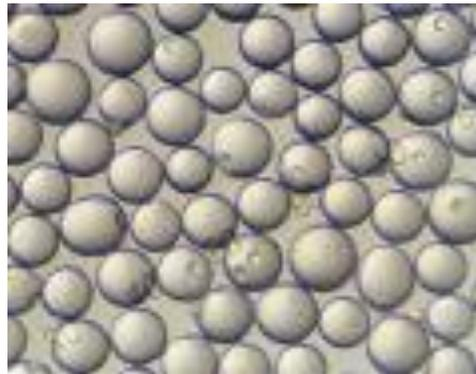
Micrograph of SH Silica 100 $\mu\text{m}$
